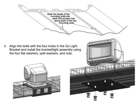
4. Center the light and tighten the hardware to secure the bracket to the lightbar.
